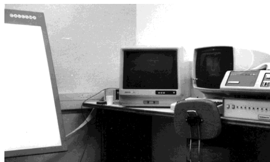
Figure 28 The graphics workstation. A part of the digitiser is visible on the left of the photo and a part of the plotter can be seen on the right. (Source: Photo collection of Mrs AD Mans)
