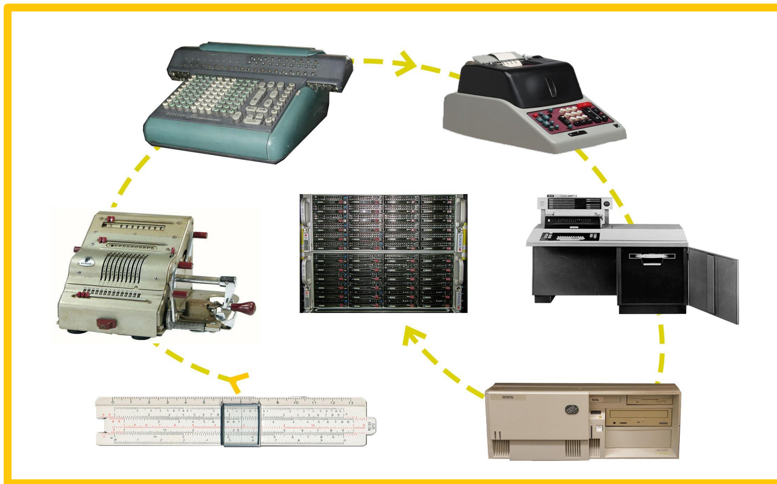
Schematic representation of the main hardware components used for calculations at the PU for CHE from the 1950s to the present time, from the slide rule to mechanical calculators,, to electrical calculators, to printing calculators, to the IBM 1130 and the mainframe era, to the first powerful servers like the IBM RS/6000, and presently the modern compact servers with multiple hard drives
