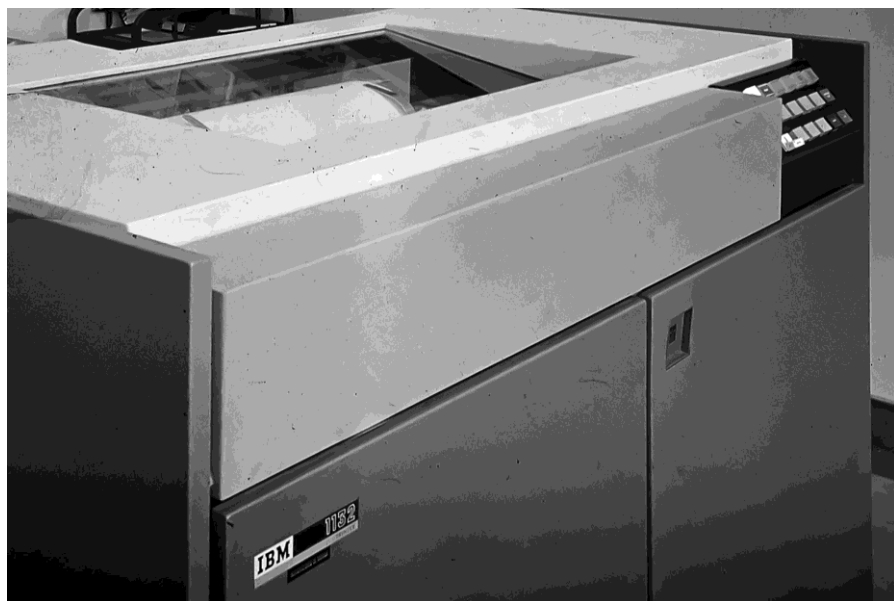
Figure 6 The IBM 1132 line printer that was later purchased. (Source: Photo collection of Mr L Smuts)
