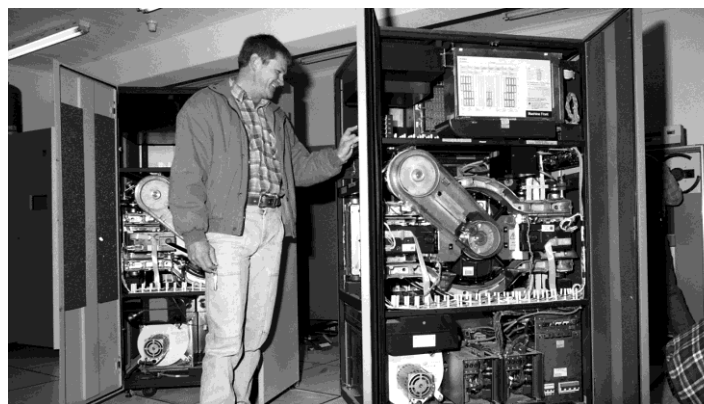
Figure 13 Mr Johan Greyling with one of the IBM 3380 disk drives during the dismantling of the mainframe computer in 1997. The IBM 3380 disk drives was an important component of the mainframe environment and had a capacity of 2.5 gigabytes. Mr Greyling was a key figure in ITM Information Systems for a long time. (Source: NWU archive)
