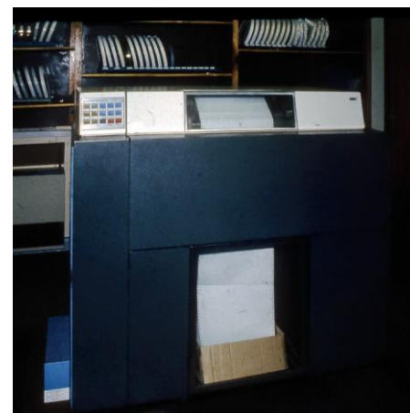
Figure 12 The IBM 1403 printer was a vital component at Task Reception. It was a fast line printer that could print approximately 1 000 lines per minute. (Source: Photo collection of Mrs AD Mans)
