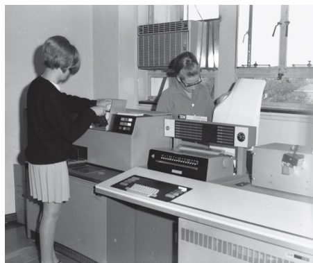
Figure 2 The University's IBM 1130 computer in 1971. The computer is in the foreground and the card reader/punch is in the background. The mechanical paper tape reader is on the far right of the photo. The identities of the two persons at the card reader are unknown. (Source: Photo collection, NWU archive)
