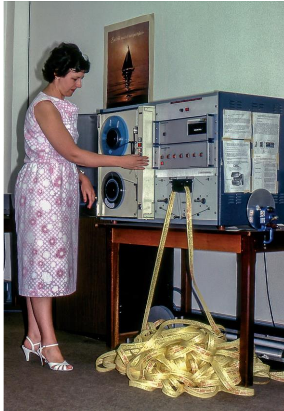
Figure 3 The media converter. On the photo, Mrs Renée Smit from the Department of Physics is transferring data from the punched paper tape to the IBM-compatible tape machine. The graph plotter is not visible on the photo. (Source: Photo collection, Mrs AD Mans)
