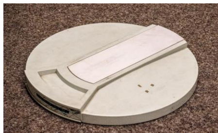
Figure 3 The IBM 1130's IBM 2310 hard drive. It had a capacity of 1 megabyte and a diameter of approximately 38 cm. (Source: Author's photo collection)
